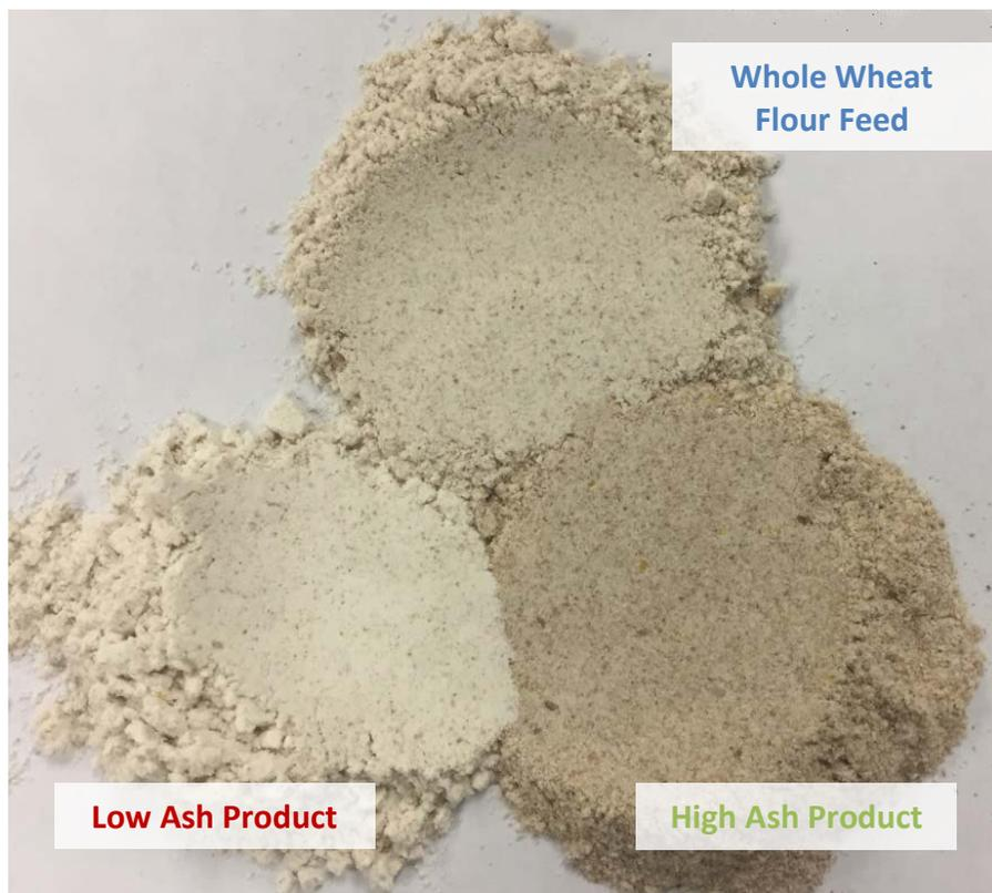
**Figure 10: Typical products recovered from the STET separation process.**
