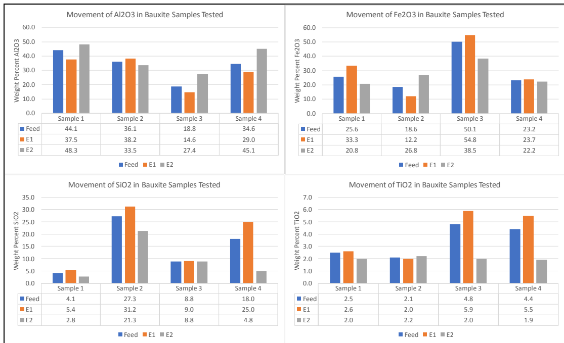
Figure 5. Bench scale separation of Al 2 O 3 , Fe 2 O 3 , SiO 2 and TiO 2 for samples tested
