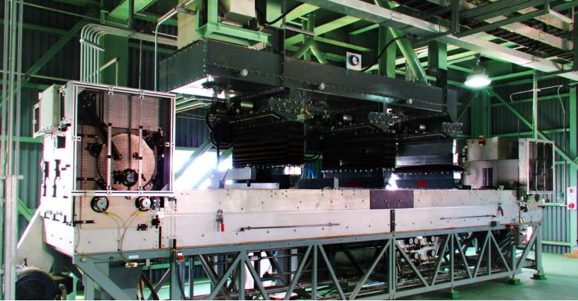
**ELECTROSTATIC EVOLUTION:** Long used to add value to fly ash from coal power, electrostatics can be a useful way to produce a higher-value DDGS in the ethanol industry. Pictured is a fly ash separator, ready to accept feed.
