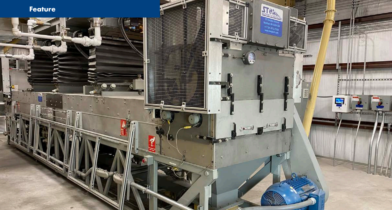
A recently installed triboelectrostatic separator.
