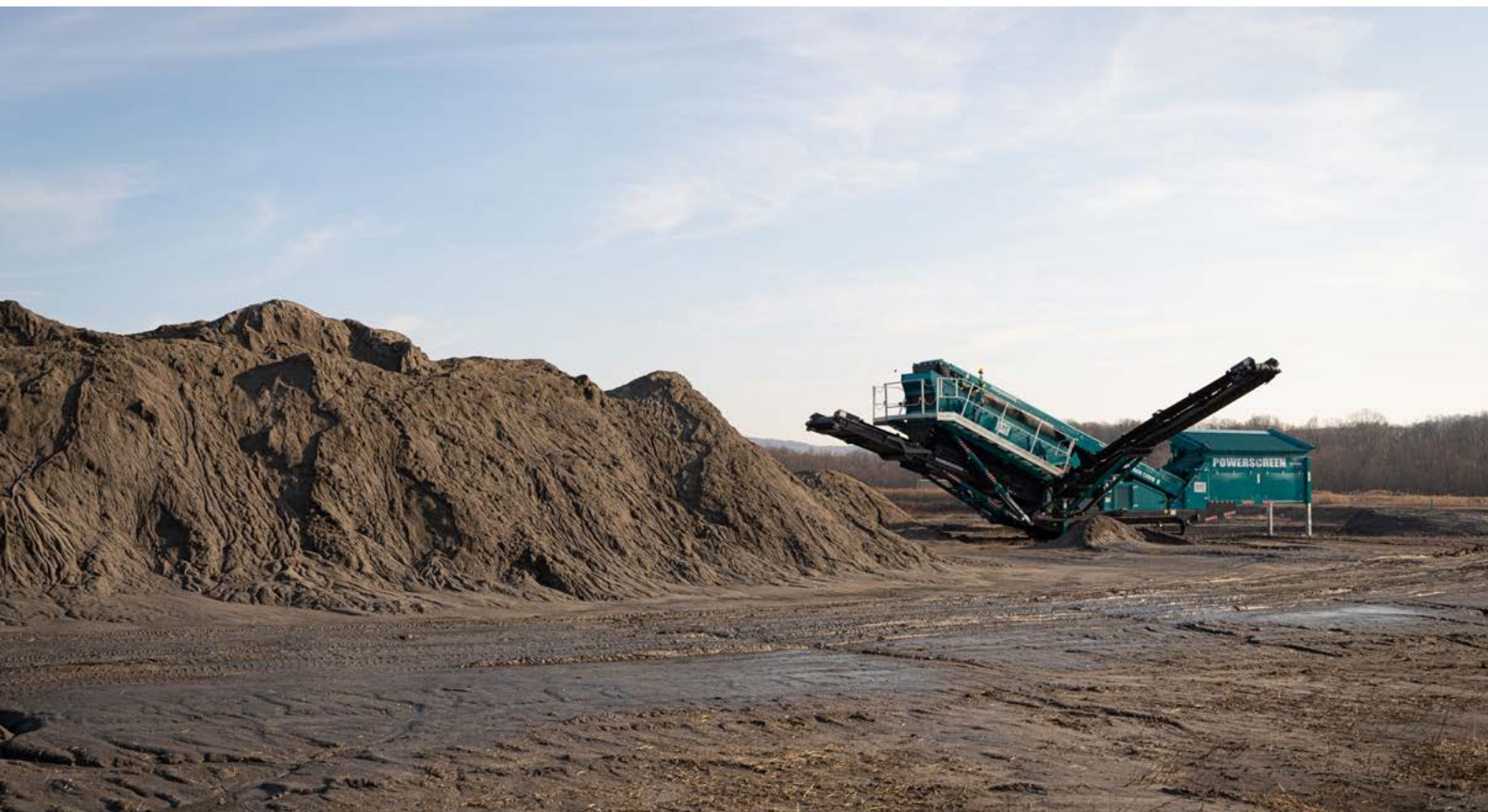
ST's coarse screening operation removing coarse debris from ponded ash. From here, the screened reclaimed ash is transported to ST's beneficiation operation for drying, particle size control, and carbon removal (i.e., separation).
